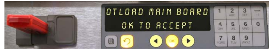
Master display with Bootload Main Board message. Press the illuminated OK.
